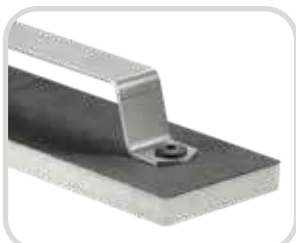
Rohacell foam + CRP top layer Pull-out force 1,300-1,700N
