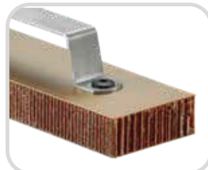
Aramid honeycomb + Aramid Pull-out force 700–1,200 N
