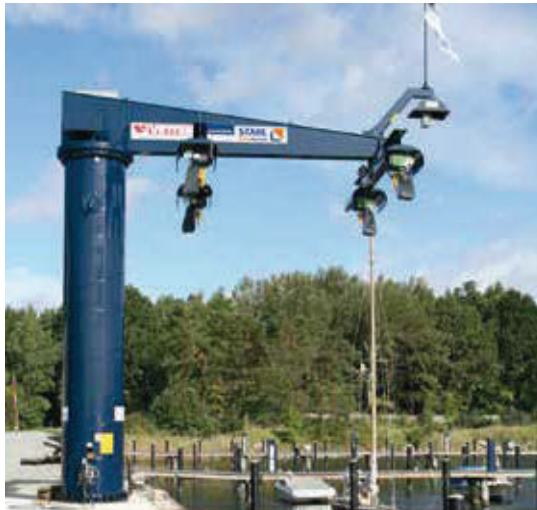
Floor mounted jib crane with four electric chain hoists ST 50
